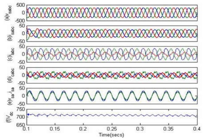
Fig. 6. Performance of UPQC for load balancing, power factor correction and current harmonic mitigation
