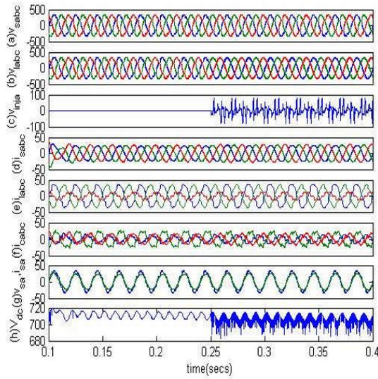
**Fig.7 Performance of UPQC for load balancing, power factor correction, current and voltage harmonic mitigation**
