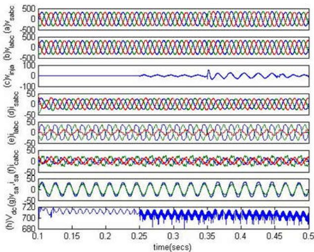
**Fig.10 Performance of UPQC for load balancing, power factor correction, current harmonic and voltage swell mitigation**
