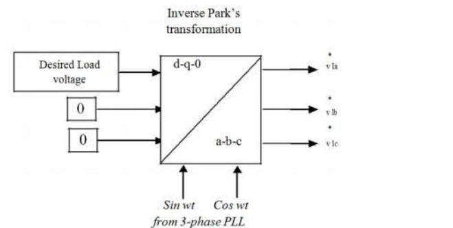
**Fig.3. Control Scheme of Series APF using SRF Theory**
