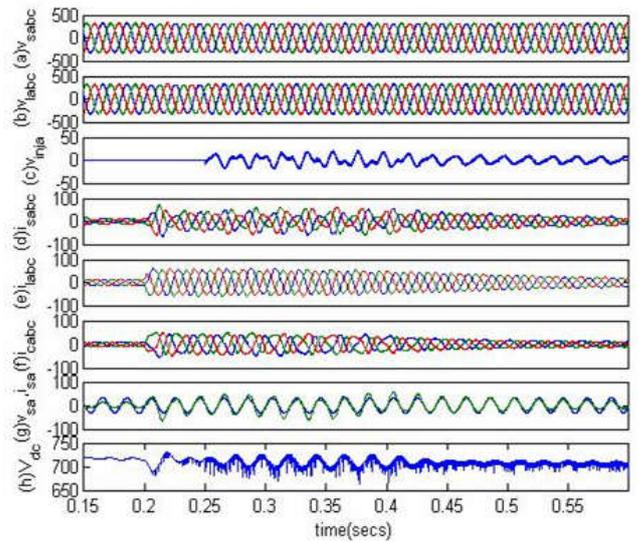
**Fig.11 Performance of UPQC for power factor correction and voltage dip mitigation**
