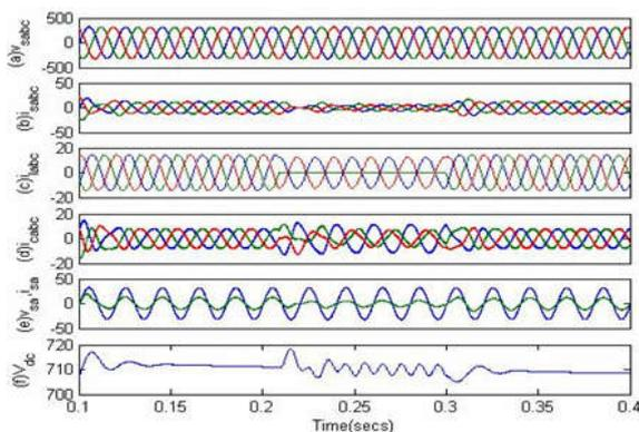
Fig. 5. Performance of UPQC for load balancing and power factor correction
