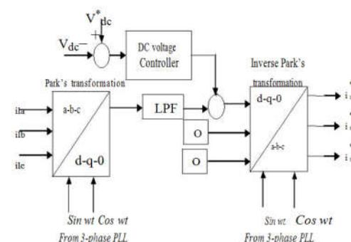
**Fig. 4. Control Scheme of Shunt APF using SRF Theory**
