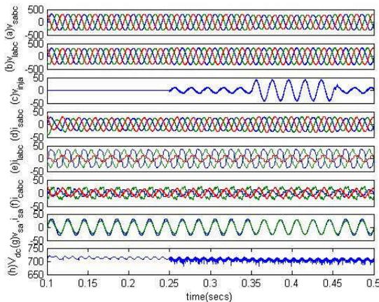
**Fig.9 Performance of UPQC for load balancing, power factor correction, current harmonic and voltage sag mitigation**
