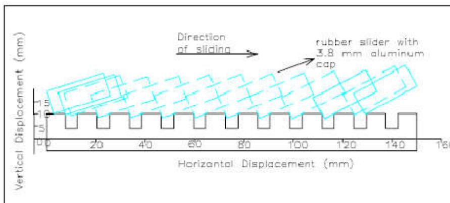
Fig. 8. Sliding path of rubber on transverse grooved surface with 5 mm groove width, 13 mm groove spacing and 6 mm groove depth (Note: Dashed lines denotes deepest penetration point of rubber into grooves)
