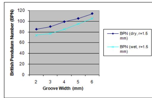
Figure 6. British pendulum measurements of rounded grooves for transverse tinning
