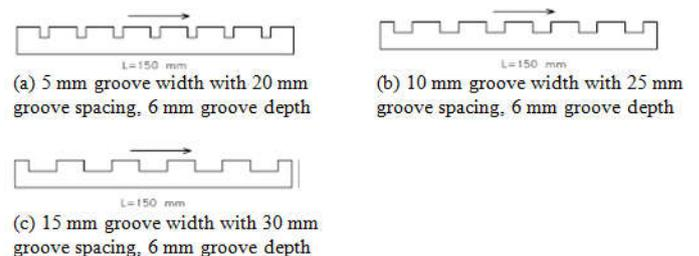
Figure 8. Transverse groove surfaces from front view with variable groove width and spacing
