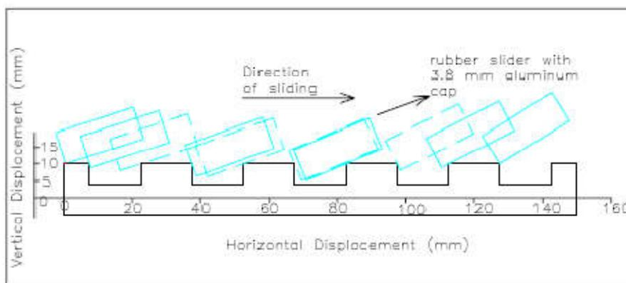
Fig. 9. Sliding path of rubber on transverse grooved surface with 15 mm groove width, 30 mm groove spacing and 6 mm groove depth (Note: Dashed lines denotes deepest penetration point of rubber into grooves)
