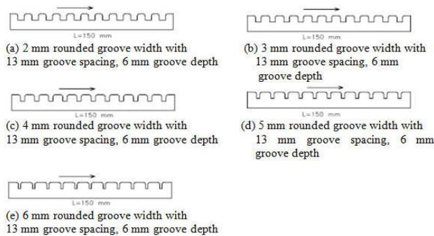
Figure 5. Transverse rounded groove surfaces from front view with variable groove width
