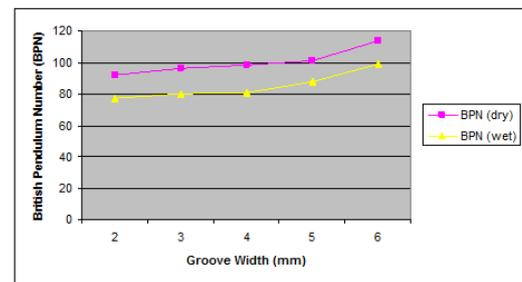
Figure 3. British pendulum measurements for transverse grooved surfaces with variable groove width, constant groove spacing and constant groove depth
