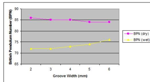
Figure 4. British pendulum measurements for longitudinal grooved surfaces with variable groove width, constant groove spacing and constant groove depth
