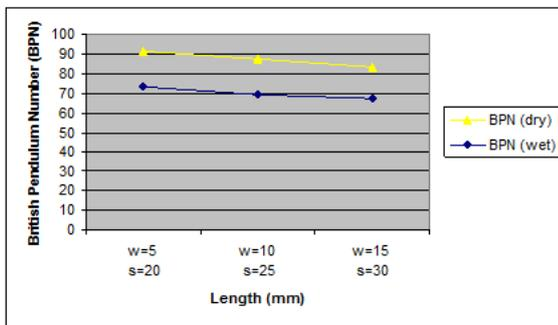
**Figure 7. British pendulum measurements of varied groove width (w) and groove spacing (s)**
