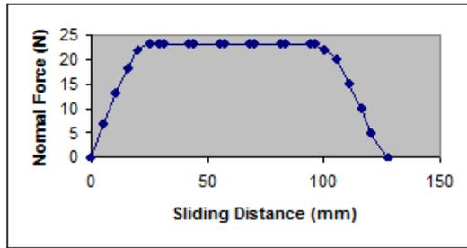
Figure 1. Static normal force for 127 mm sliding distance
