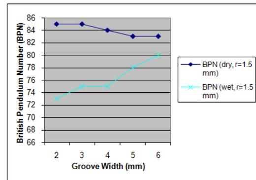
Figure 7. British pendulum measurements of rounded grooves for longitudinal tinning
