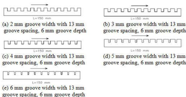
Figure 2. Transverse grooved surfaces from front view with variable groove widths (Note: Arrows denotes sliding direction)
