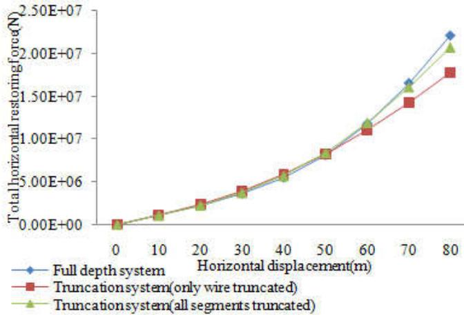
Fig. 7. Total horizontal restoring force results comparison
