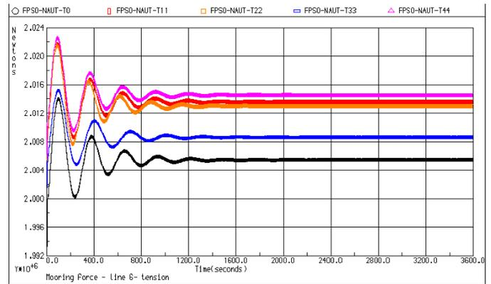
Fig. 10. Time domain response curves of 6-th mooring line top tension
