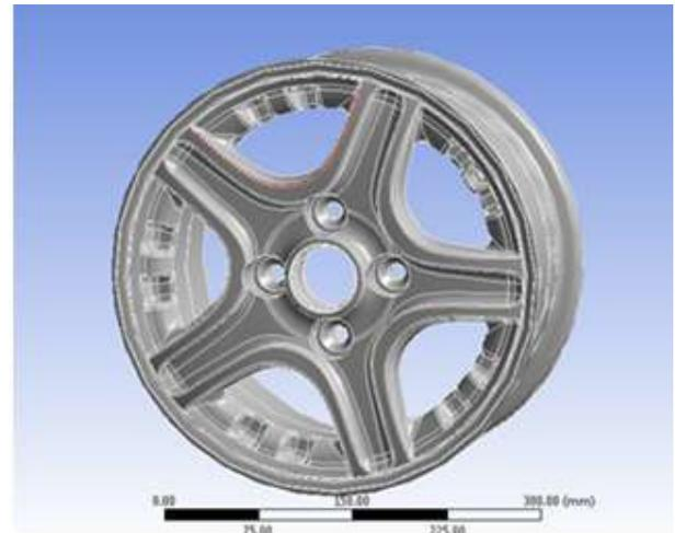
Figure 1. 3D model of Aluminium Alloy Wheel
