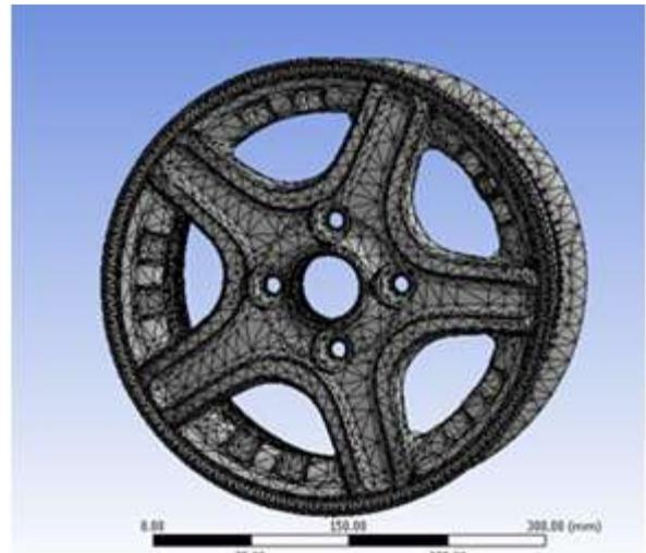
Figure 2. Meshing of Aluminium Alloy Wheel
