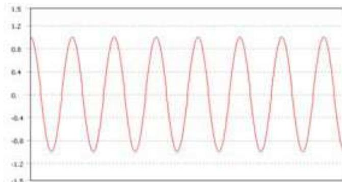
Figure 8. Constant amplitude fully reversed
