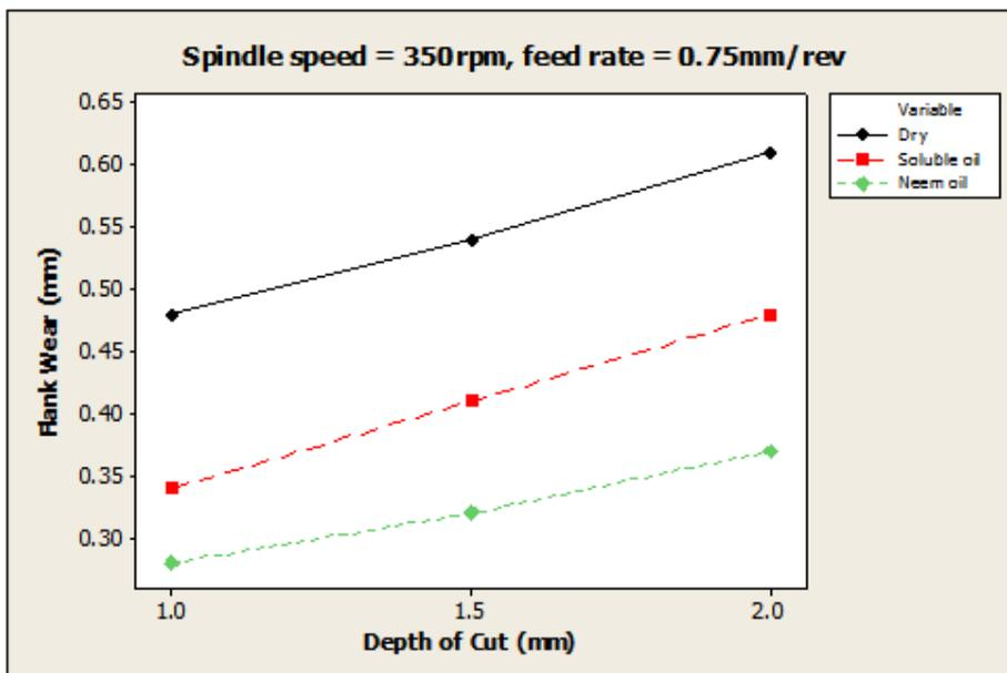
Figure 6. Effect of depth of cut on flank wear (N = 350rpm, f = 0.75 mm/rev)
