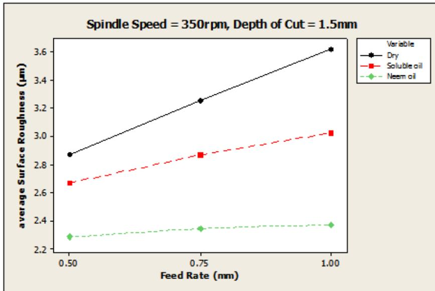
Figure 2. Effect of feed rate on surface roughness (N = 350rpm, d = 1.5mm)
