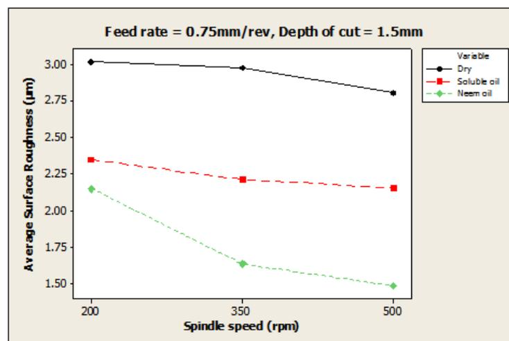
Figure 1. Effect of spindle speed on surface roughness ( $f = 0.75\text{mm/rev}$ ,  $d = 1.5\text{mm}$ )
