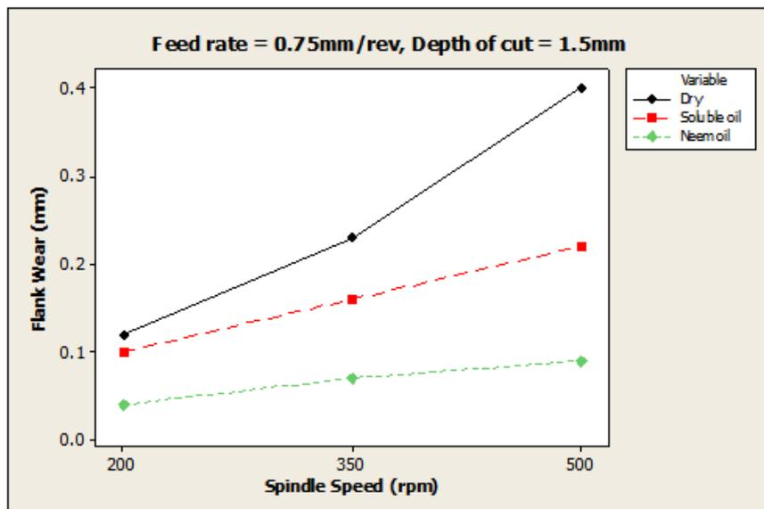
Figure 4. Effect of spindle speed on flank wear (f = 0.75mm/rev, d = 1.5mm)
