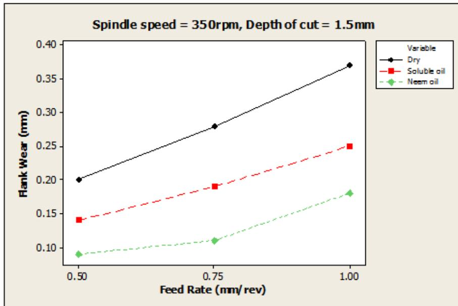
Figure 5. Effect of feed rate on flank wear (N = 350rpm, d = 1.5mm)
