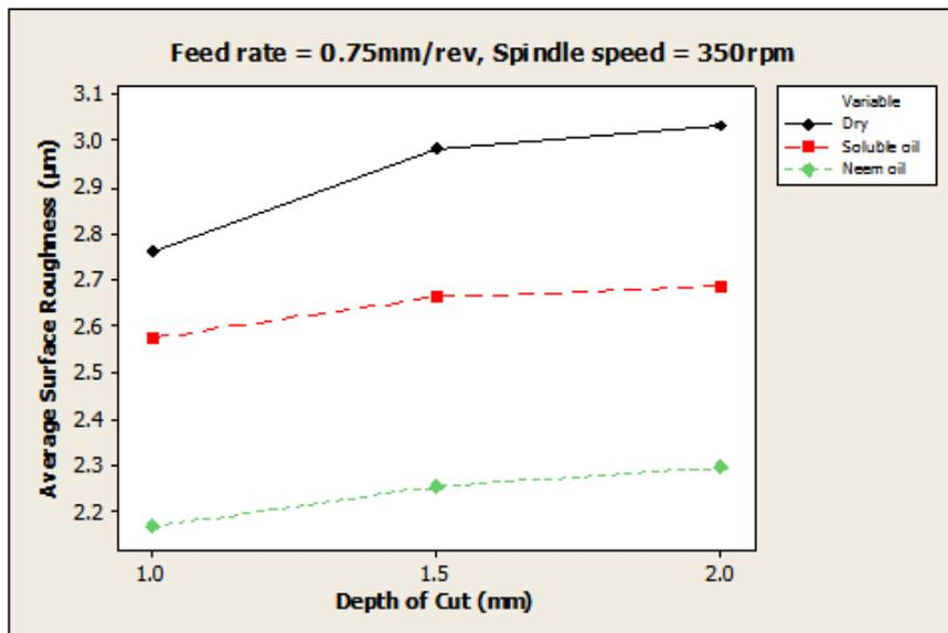
Figure 3. Effect of depth of cut on surface roughness (f = 0.75mm/rev, N = 350rpm)
